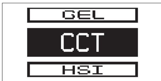
2.2.1 Press the INT button to select CCT mode to adjust the color temperature of the light from 2000K-10000K.
