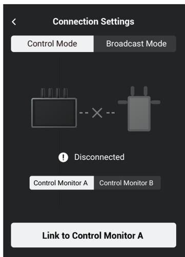
2. Using Ronin 4D: to start linking, hold the link button on the Ronin 4D Video Transmitter or go to menus on the Ronin 4D High-Bright Main Monitor, tap Transmission, and Link Device. The linking status indicator on the video transmitter blinks red and green alternately, indicating the device is linking.
