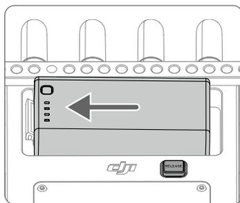
Press and hold the WB37 battery release button and push the battery in the opposite direction to remove it.
