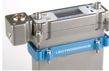
Thread two short screws through the recessed tabs on the adapter and slide it onto the receiver housing. Thread two short screws through the tabs on the receiver flange as shown.
