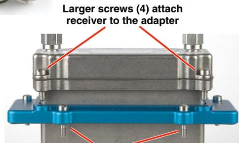
Larger screws (4) attach receiver to the adapter
