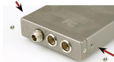
Panels are held in place by two Phillips head screws on the sides of the housing.
