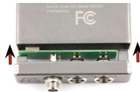
Carefully align the mating connectors and gently slide the panel straight into the housing until the screw holes align with the housing.
