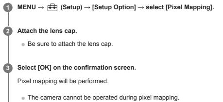
• The camera will restart when pixel mapping is complete.
