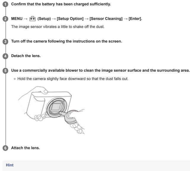
• For how to check the amount of dust on the image sensor, and for further details on cleaning methods, please refer to the following URL.
