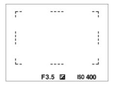
• When you use a zoom function other than the optical zoom, the [ Security Focus Area] setting is disabled and the focusing frame is shown by the dotted line. The AF operates with priority on and around the center area.
