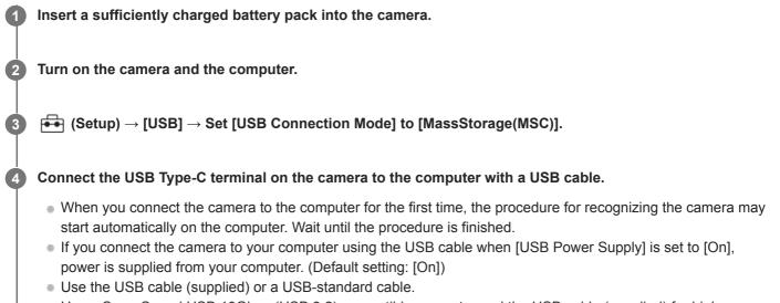
Use a SuperSpeed USB 10Gbps (USB 3.2)-compatible computer and the USB cable (supplied) for higherspeed communications.
