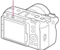
Press the MODE button, use the control wheel to select the desired shooting mode, and then press the center of the control wheel.
